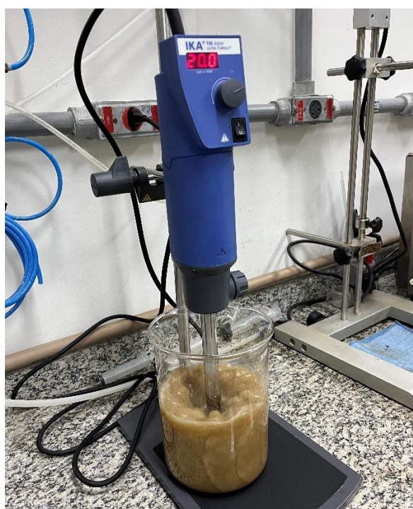
Figure 19 - Preparation and homogenization of oily wastewater influent using high-speed ULTRA-TURRAX mixing.
