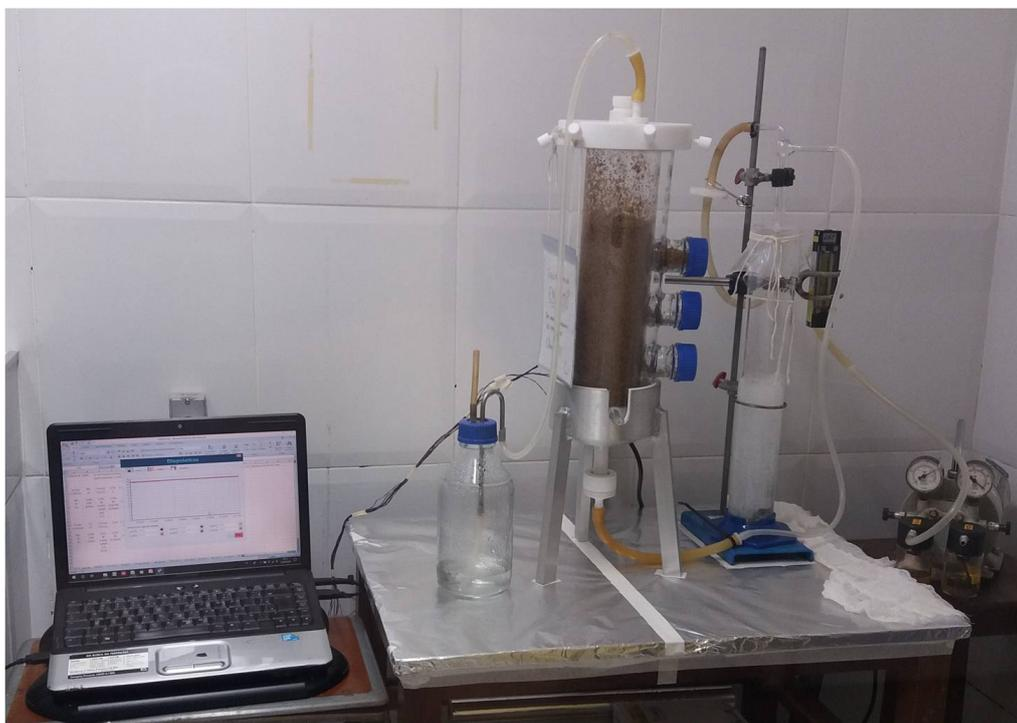
Figure 4.1: Fixed-bed bioreactors used for solid-state fermentation. In the center, the insulated packed-bed bioreactor with a vacuum-sealed jacket is filled with soybean hulls. The volumetric cylinder used to humidify the air before entering the bioreactor is shown in the right. A schematic drawing of the bioreactor system is also shown in Figure 4.7.
